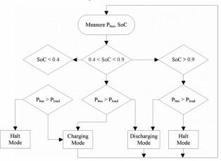
Fig. 5. Bidirectional Convertor Control Algorithm [5]
